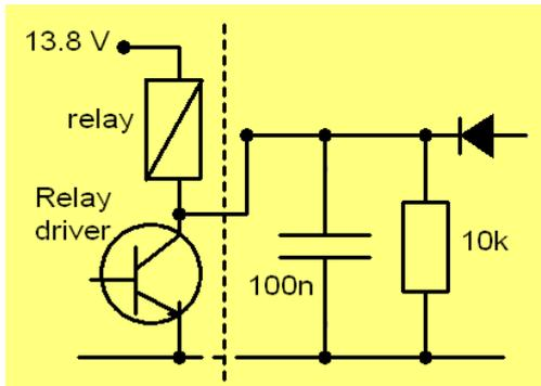
Add Mutant to a relay driver to expand the switching capability. Check the relay is adequately suppressed.
