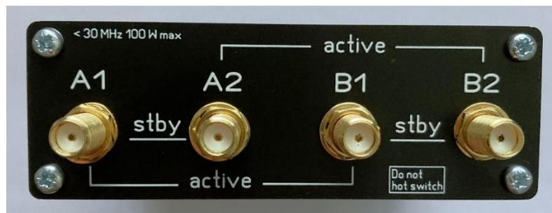
When the RF control line is inactive, or the unit is unpowered, A1 is connected to A2, and separately, B1 is connected to B2.
