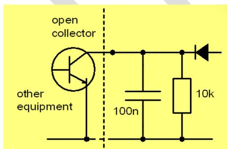
Many transceivers and some receivers have undedicated open collector outputs. Mutant could be used to swap antennas or insert an attenuator for instance.
